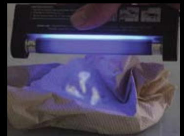
Longwave UV lights are useful in viewing invisible stains at the crime scene, as well as theft detection powders and pastes.
