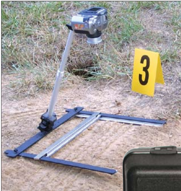
DEPS100 (above) is used to take an evidential photo of a tire track (resultant photo shown below).
